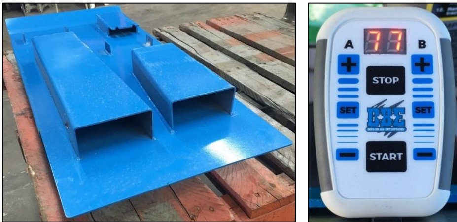
New dual fan plenum & controller for fan speed adjustment.
